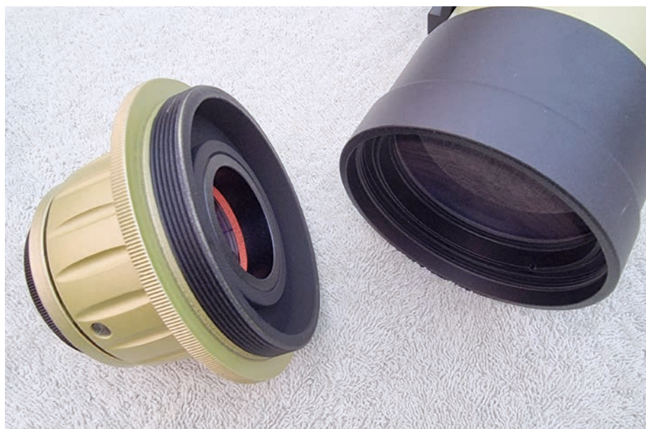
▼ The etalon simply unscrews from the main refractor body. Image: Steve Ringwood.
